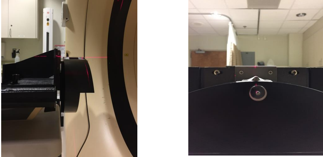
Fig. 4.6 An experimental setup for scatter signal measured is shown. A tungsten rod was placed on top of calibration phantom
